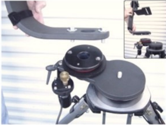
Remove 2 screws and the head frame detaches from the pan base.
