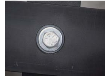
NOTE: Make sure that the channel's big hole, fits over the nylon washers.
