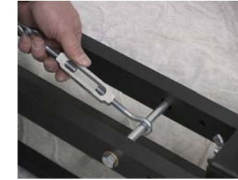
Hook the cable to cross barn near the end of the extension. Tighten the turn buckles to strengthen & straighten the Jib.
